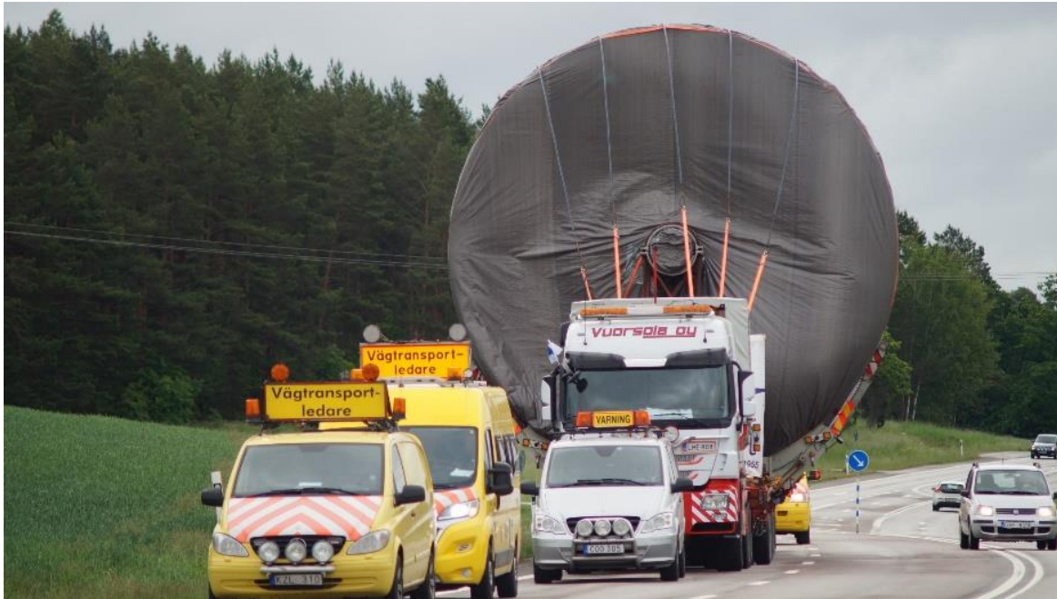
A Yankee cylinder of 160 tons on the move from Tervasaari to Skärblacka
